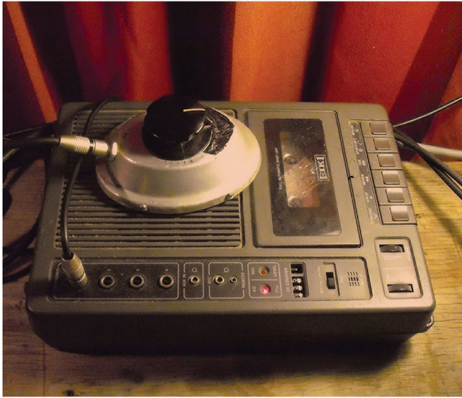
Figure 10. Larsen-Jensen's 'pie-dish' oscillator used with tape-machine amplifier (Reprinted with permission from Felix Larsen-Jensen, 2012).
